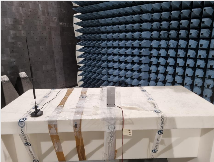
Photograph 3: EUT test setup in the semi anechoic chamber, measurement <1 GHz, close up view
