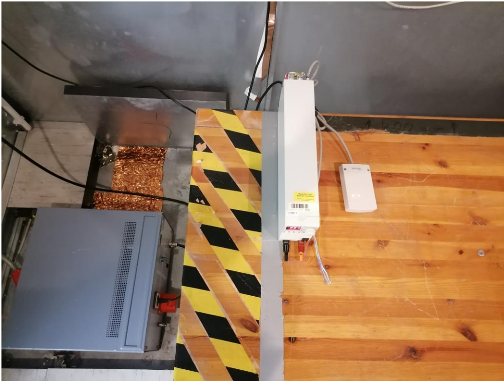
Fig. Mea.: 1 : Conducted Emission (Mains) Test Setup 1 1.01
