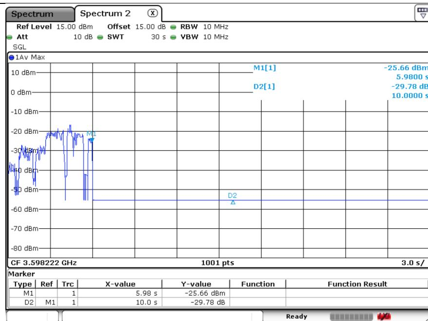
[Step 5] Configure SAS granted CBSD to operate at frequency 3650-3690MHz & power level 7dBm/MHz
