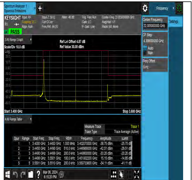
NTNV-N78-3450-3550-PC2-30-100-M-DFT-QPSK-Edge_1R B Left-Ant5-PASS
