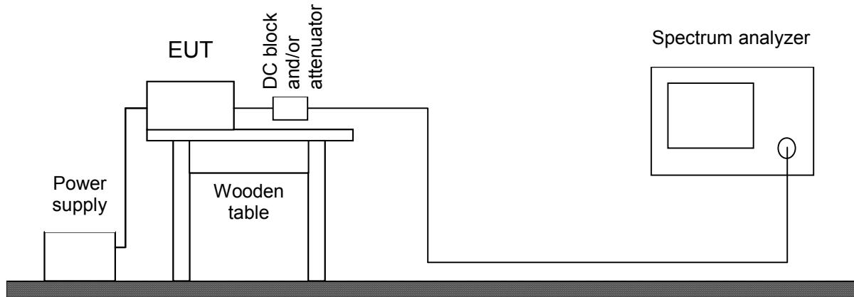
Test instruments used for conducted measurements:
