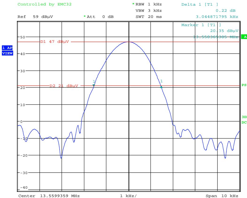
Occupied Bandwidth (-26 dB): **3.04 kHz**
