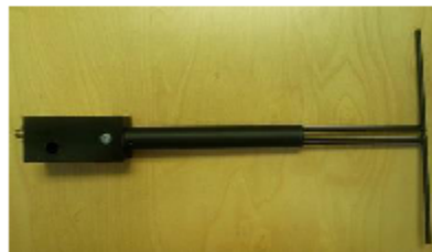
Figure 1 – MVG COMOSAR Validation Dipole
