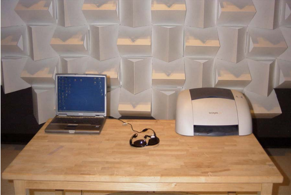
RADIATED EMISSIONS TEST SET UP
