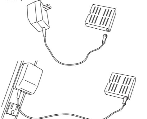
2. Plug in the power supply into the 115V-120V wall socket.
