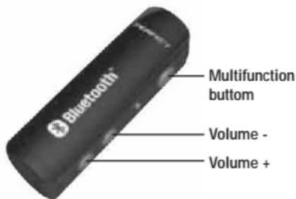
**Battery dead.** When the BT-807 battery has almost run down, the light will flash red and a beep will be heard in the earpiece. Please change battery.
