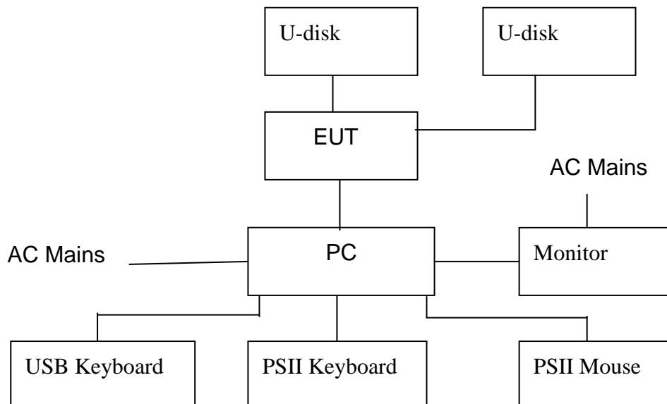
(EUT: PS3 Wireless Controller with Mini Keyboard)
