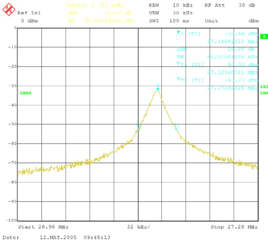
**The results: The unit does meet the FCC Part 15 C Section 15.227 requirements.**
