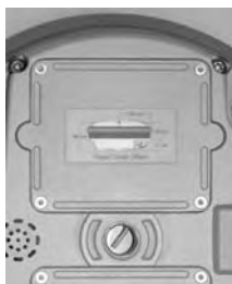
Figure 6: Mounting Socket and Phase Center Offset Label
