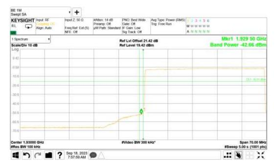
Antenna B - Modulation NR: QPSK - Carrier Bandwidth NR: 35.0 MHz - Channel Position T
