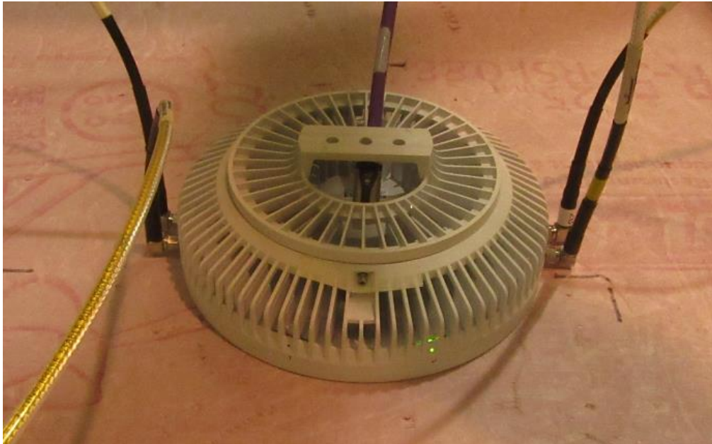
Figure 1: The EUT with four external RF ports
