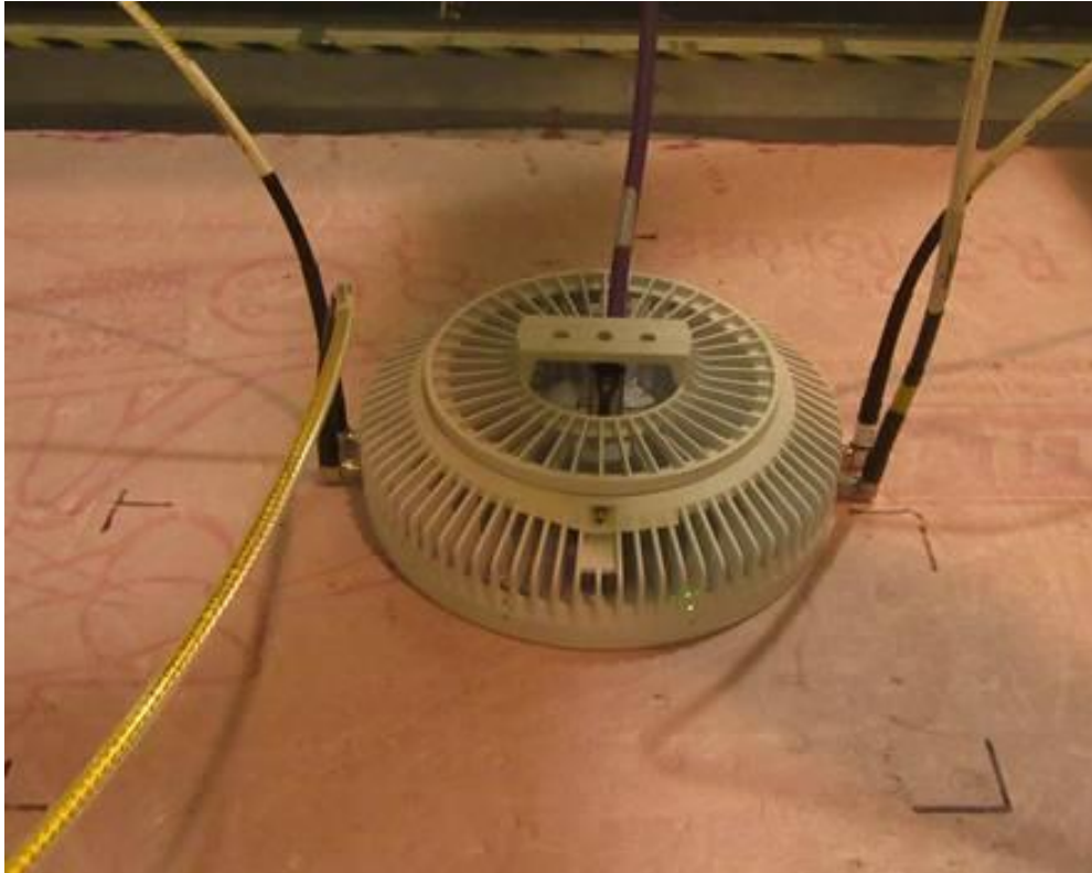
Figure 38: Setup for RE tests - Close up
