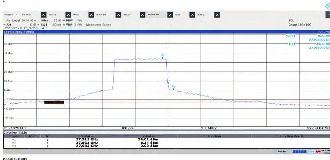
Diagram 20b: Pre scan 27.625 – 28.225 GHz, Symbolic name: TL 100 , EIRP Vertical polarization
