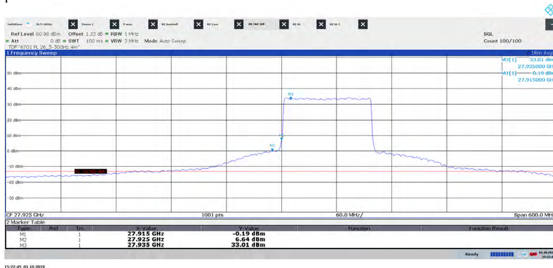
Diagram 21a: Pre scan 27.625 – 28.225 GHz, Symbolic name: BH 100 , EIRP Horizontal polarization
