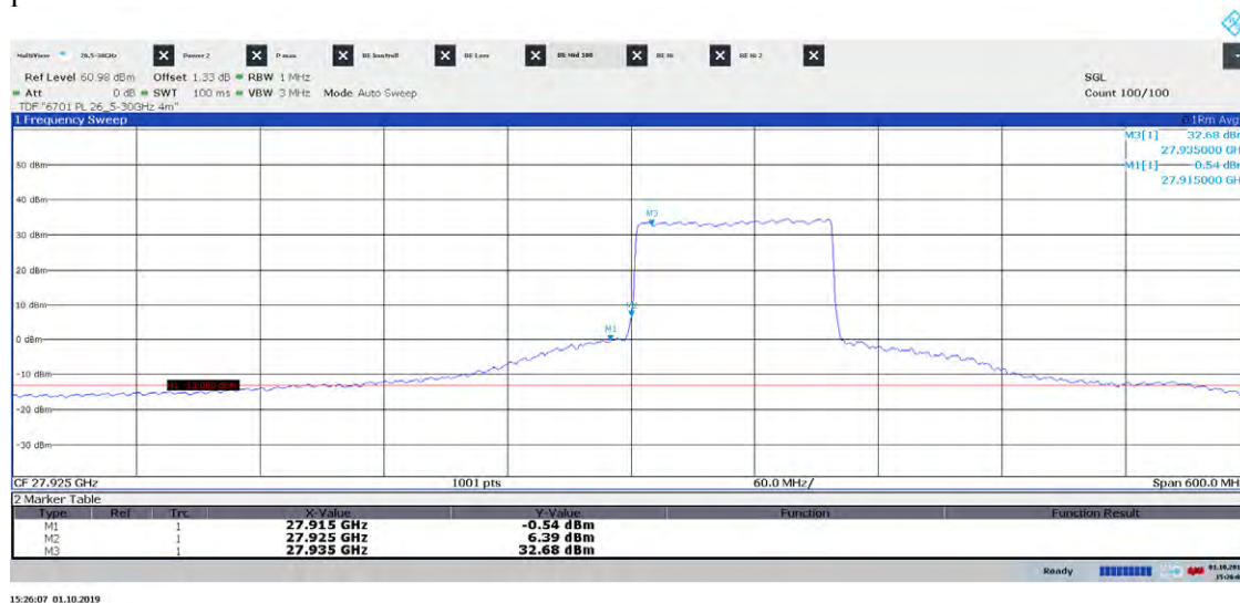
Diagram 21b: Pre scan 27.625 – 28.225 GHz, Symbolic name: BH 100 , EIRP Vertical polarization
