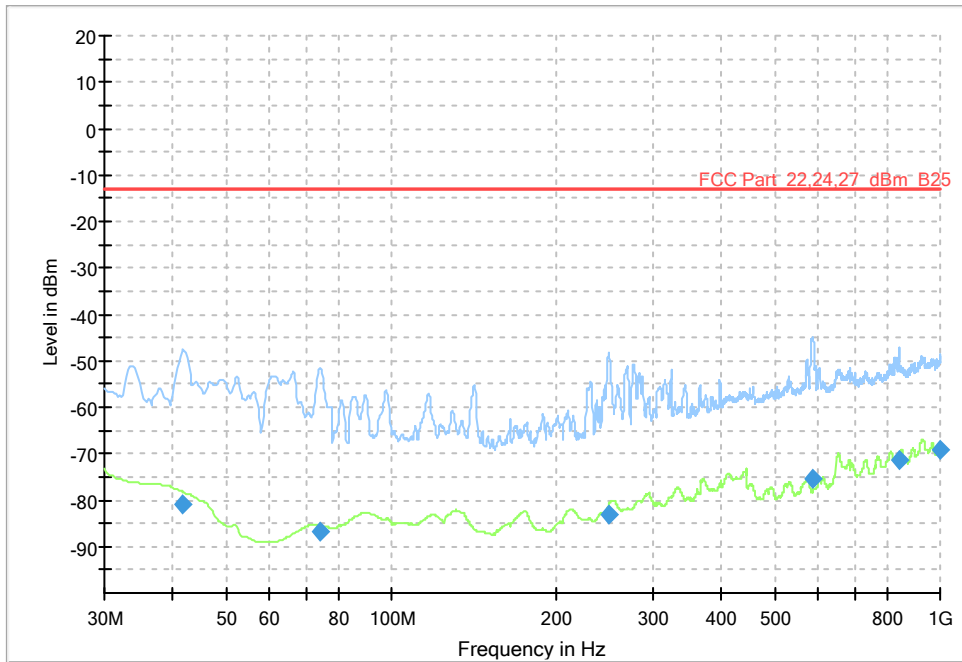
Diagram, Peak and average overview sweep, 30 – 1000 MHz at 3 m distance, configuration C2.
