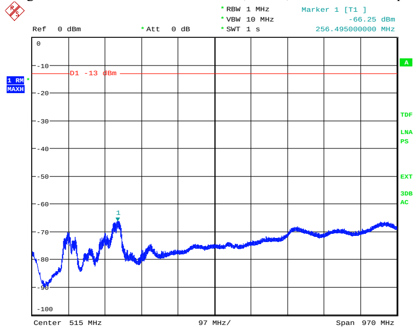
Diagram 2.2a: Pre scan 30 – 1000 MHz, M8 100 , EIRP Horizontal polarization
