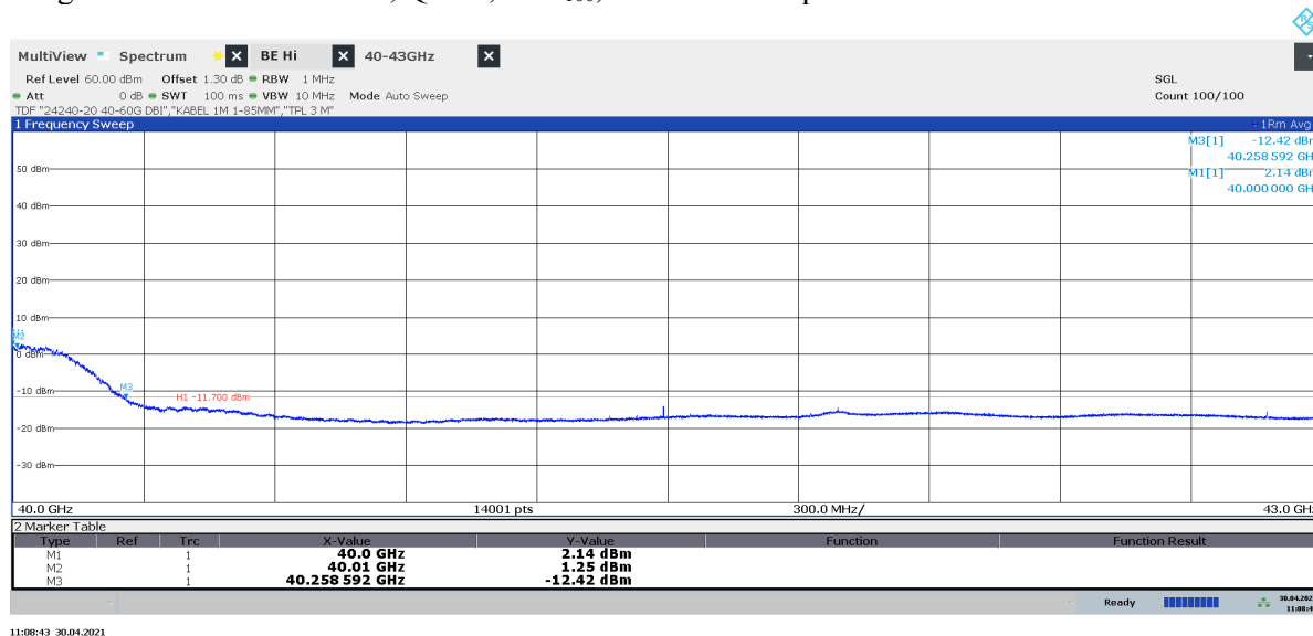
Diagram 2.22d: 40 – 43 GHz, QPSK, TH 8100 , EIRP Vertical polarization
