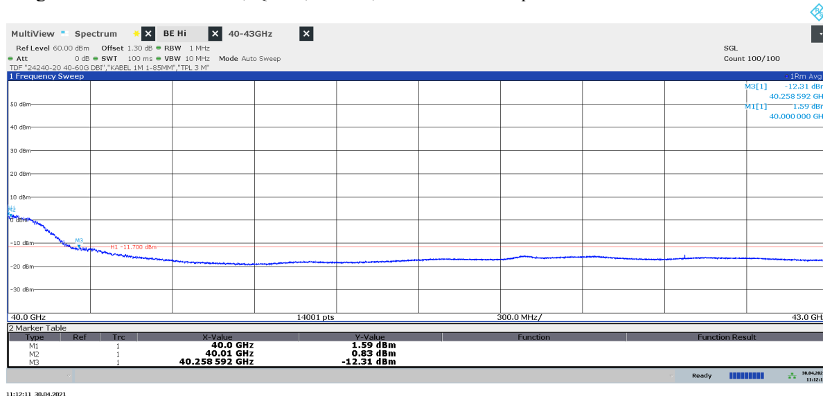
Diagram 2.22c: 40 – 43 GHz, QPSK, TH 8100 , EIRP Horizontal polarization
