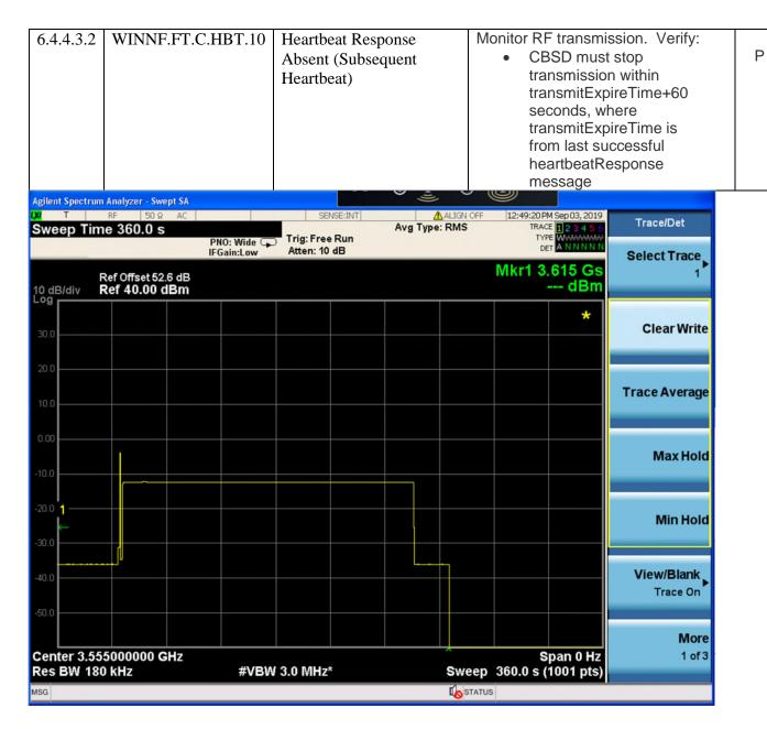
Test Harness logs and timing on graph was verified, the EUT passed the requirement.
