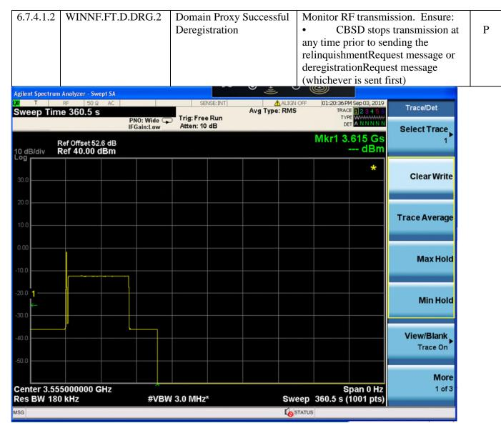
Test Harness logs and timing on graph was verified, the EUT passed the requirement.
