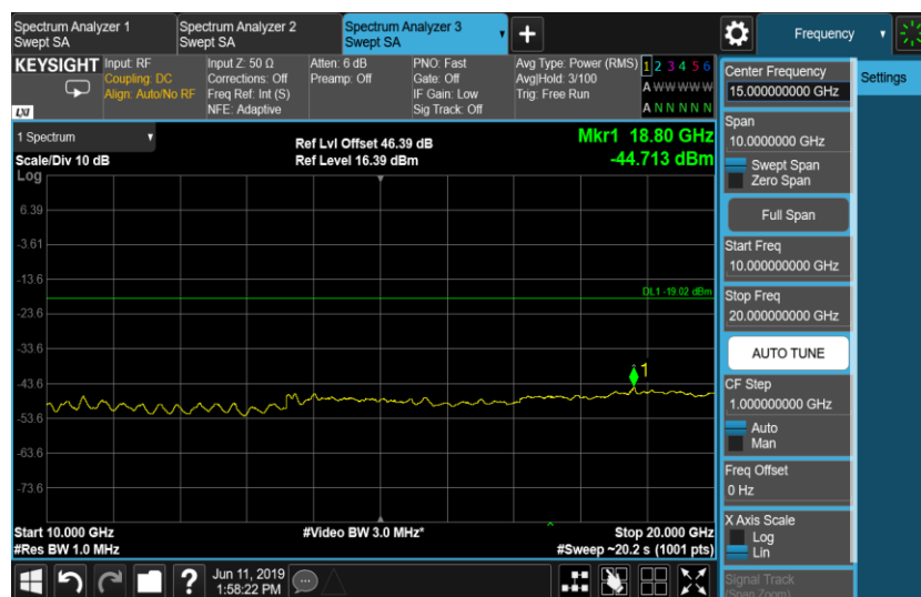
Configuration LTE+NB-IoT-MIMO-MC-1 (1LTE QPSK+1SA QPSK)
