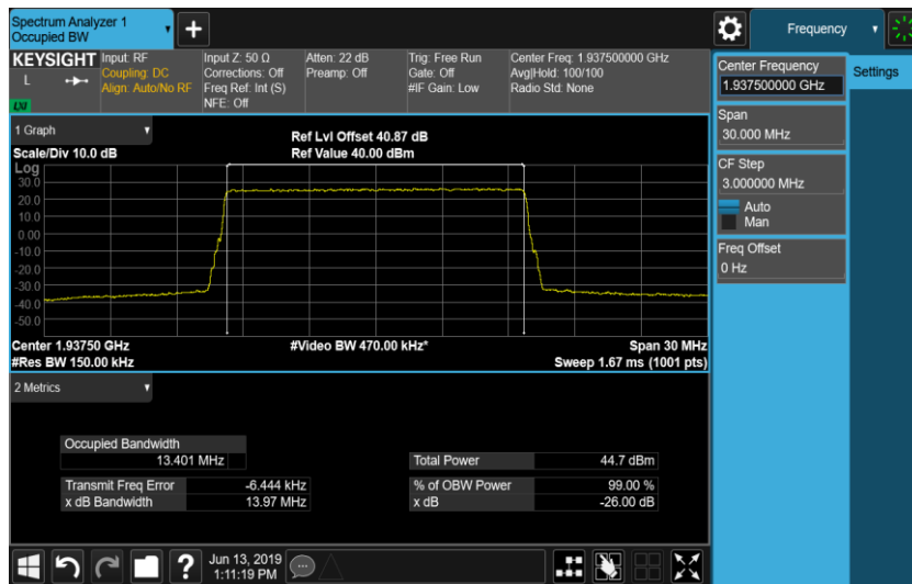
Port B, QPSK/15.0MHz Channel Position B
