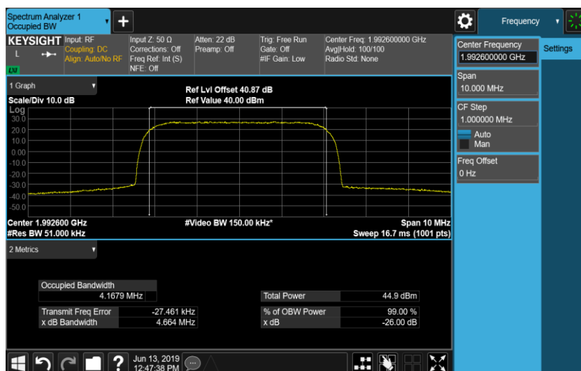
Port B, 64QAM/5.0MHz Channel Position T
