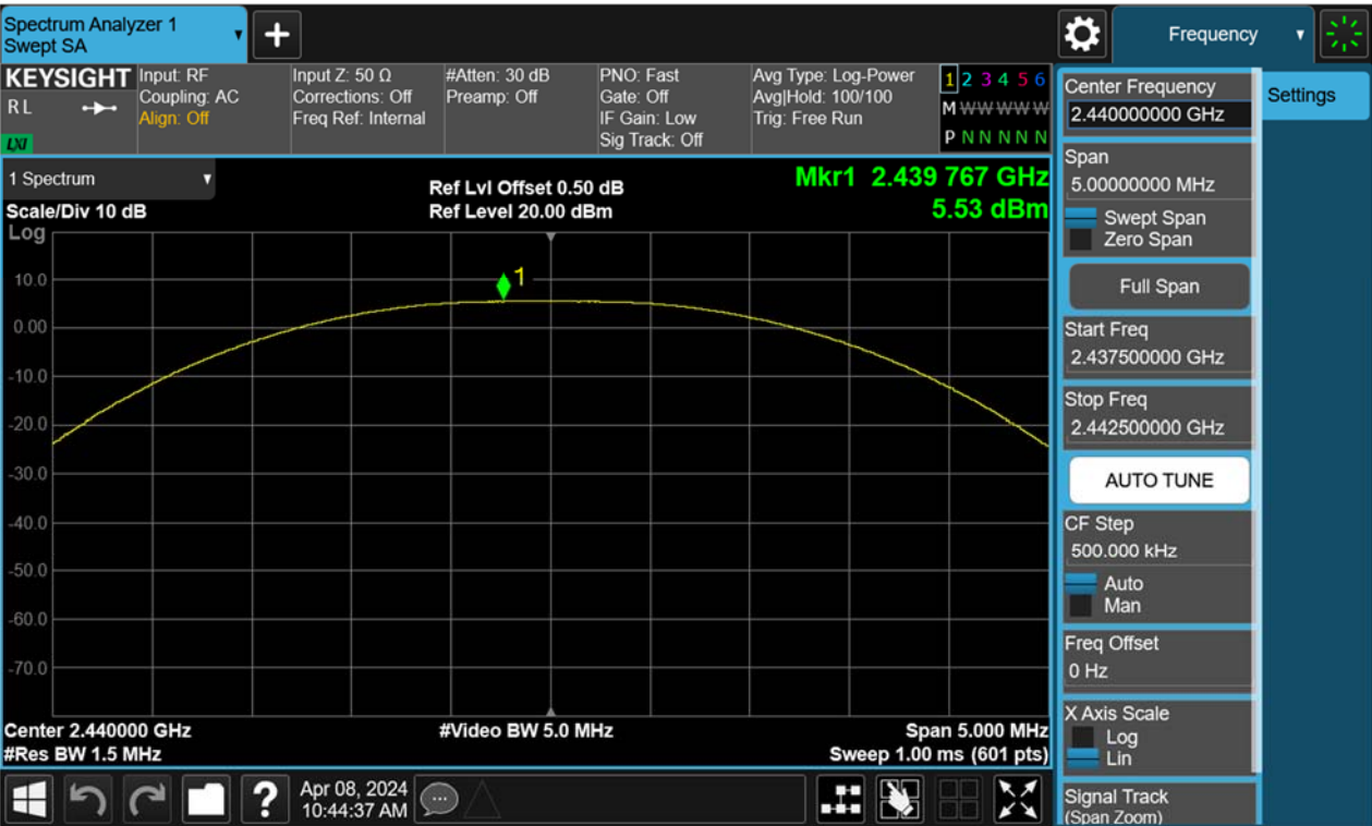
Figure 14: Peak Output Power, 2440MHz, BLE-1Mbps
