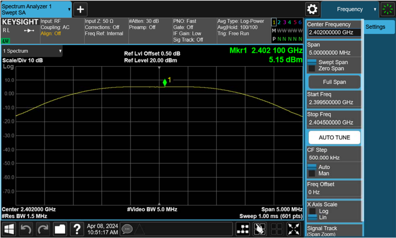
Figure 16: Peak Output Power, 2402MHz, BLE-2Mbps
