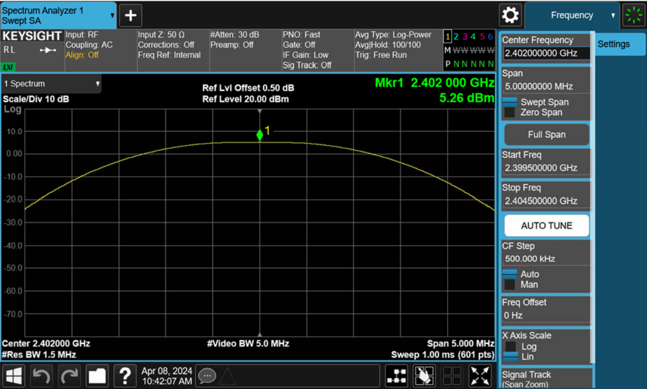
Figure 14: Peak Output Power, 2440MHz, BLE-1Mbps
