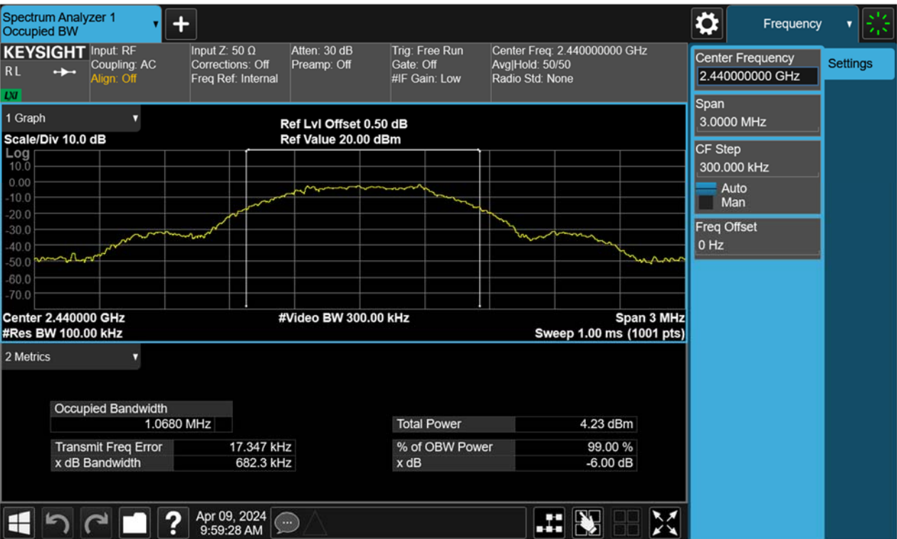
Figure 26: 6dB Bandwidth, 2440MHz, BLE-1Mbps
