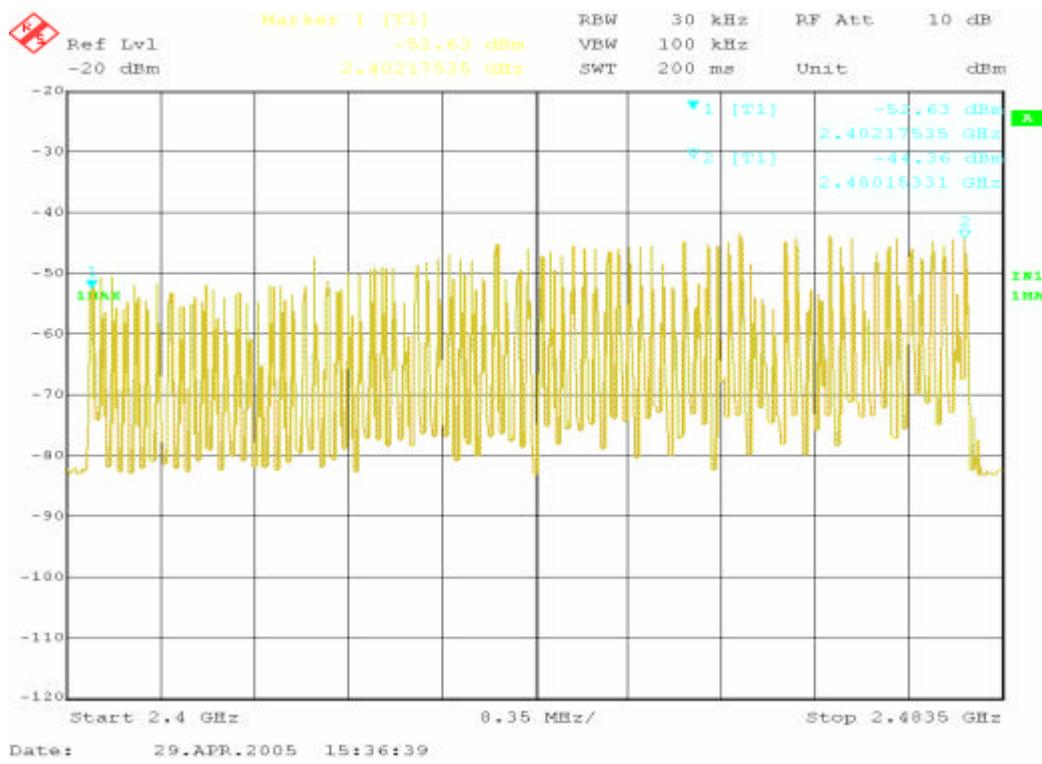
**5.3.5 Occupied Bandwidth & Carrier Frequencies Separated**
