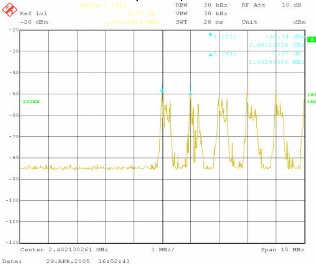
**2. Middle Channels: Carrier Frequencies Separated**
