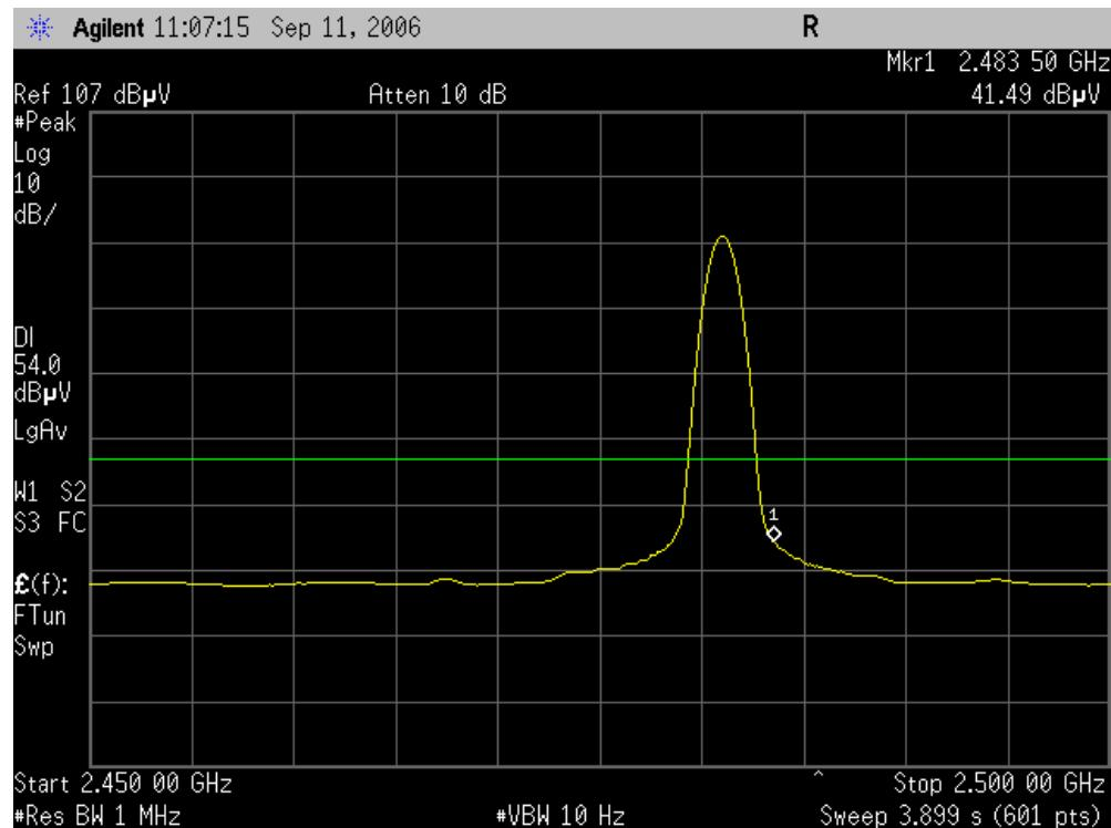
**2400 MHz Band Edges (CH-Low)****Detector mode: Peak****Polarity: Vertical**
