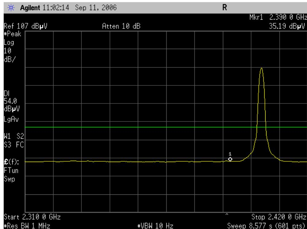
**Band Edges (CH-High)****Detector mode: Peak****Polarity: Vertical**
