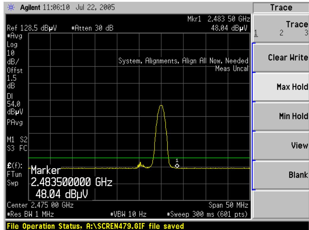
**Detector mode: Peak      Polarity: Horizontal**
