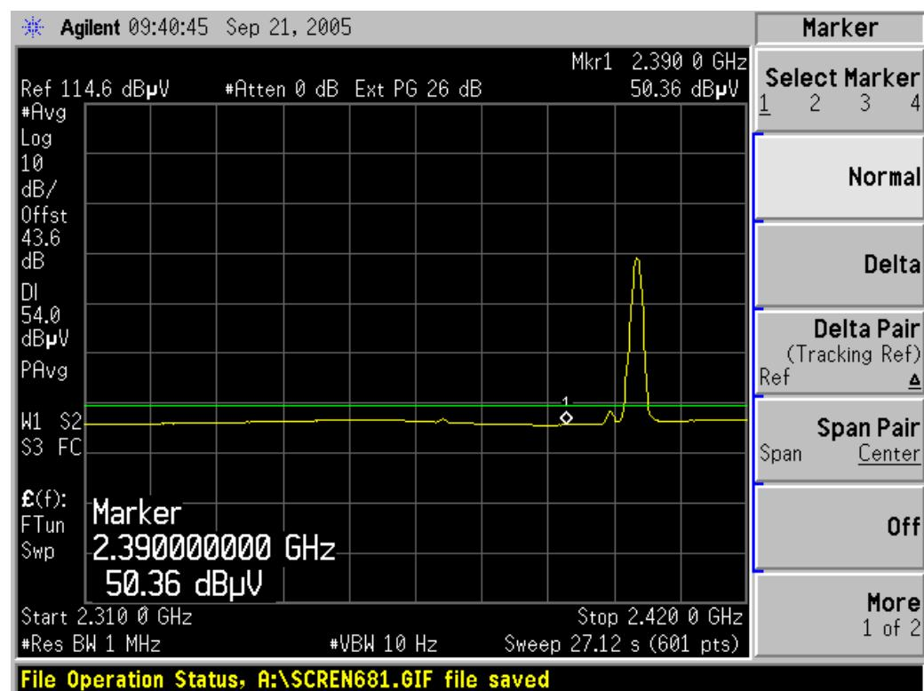
Detector mode: Peak      Polarity: Horizontal
