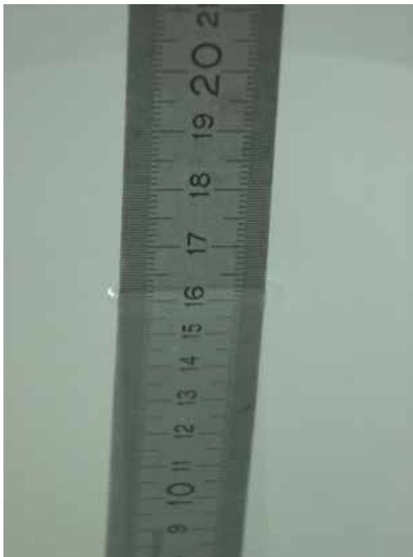
Fig. 25: Liquid depth for GPRS 1900 and WCDMA II Body measurements.
