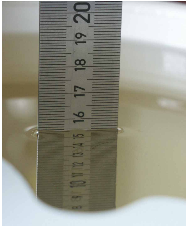
Fig. 24: Liquid depth for GPRS 850 and WCDMA V Body measurements.
