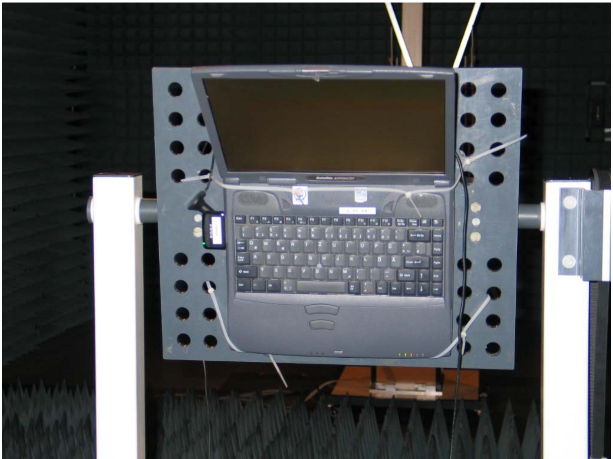
Photo 3: Setup for radiated tests
