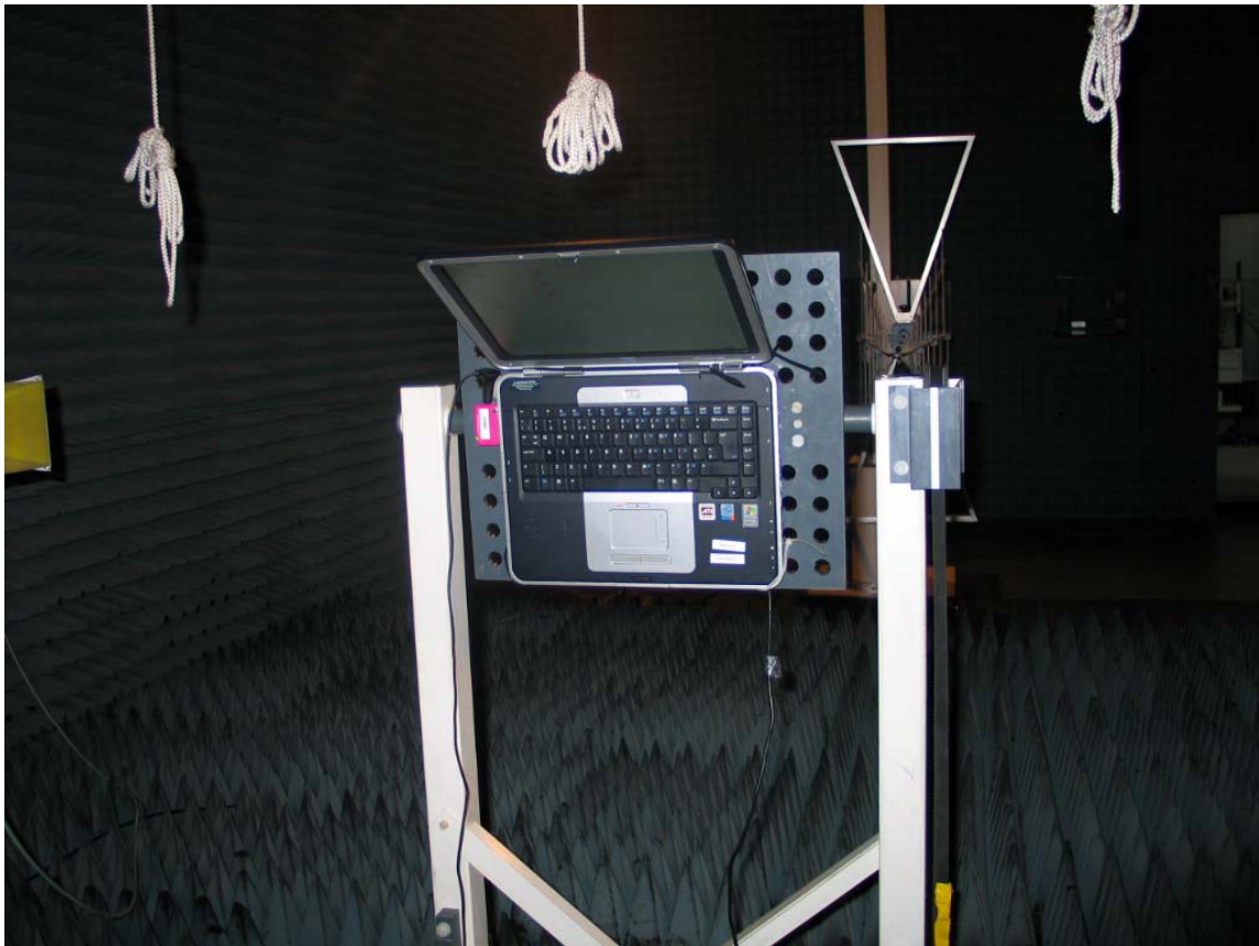
Photo 5: Setup for radiated tests
