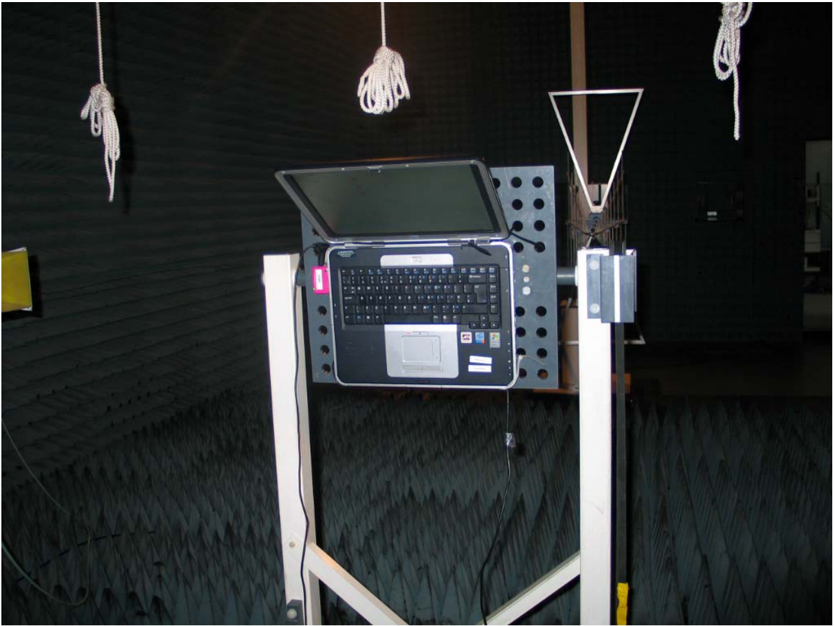
Photo 5: Setup for radiated tests
