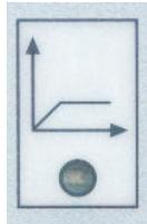
By releasing the + and - keys when this symbol is illuminated, we can access the **Strategy** mode.
