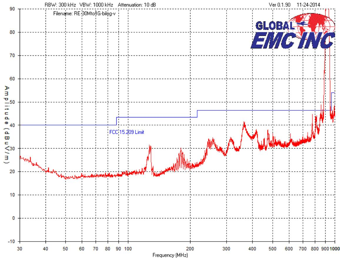
Note the device was scanned at low, middle and high channel, and the results shown above are worst case results.
