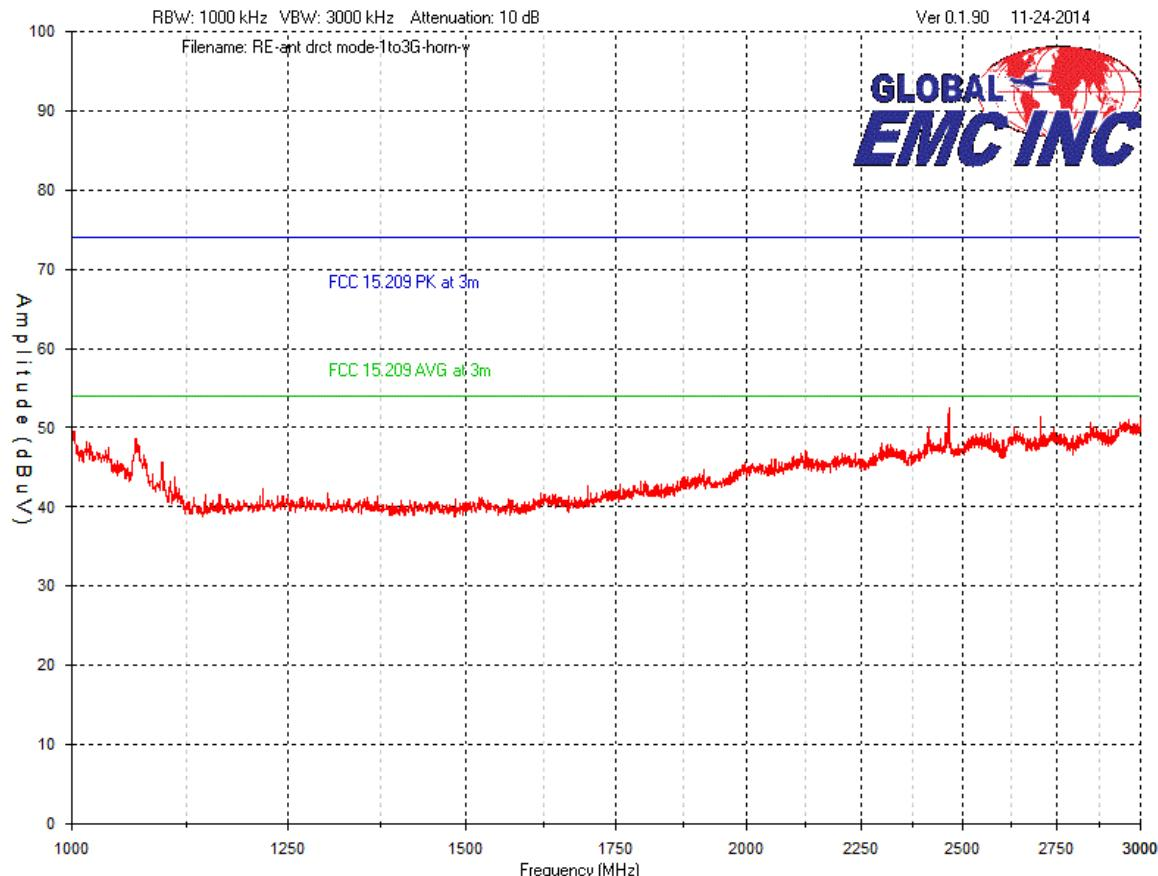
Note the device was scanned at low, middle and high channel, and the results shown above are worst case results.
