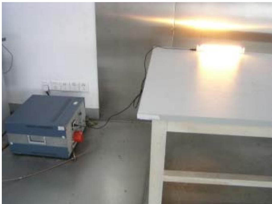
EDFT5-108L-MEO: Conducted Emission – Side View
