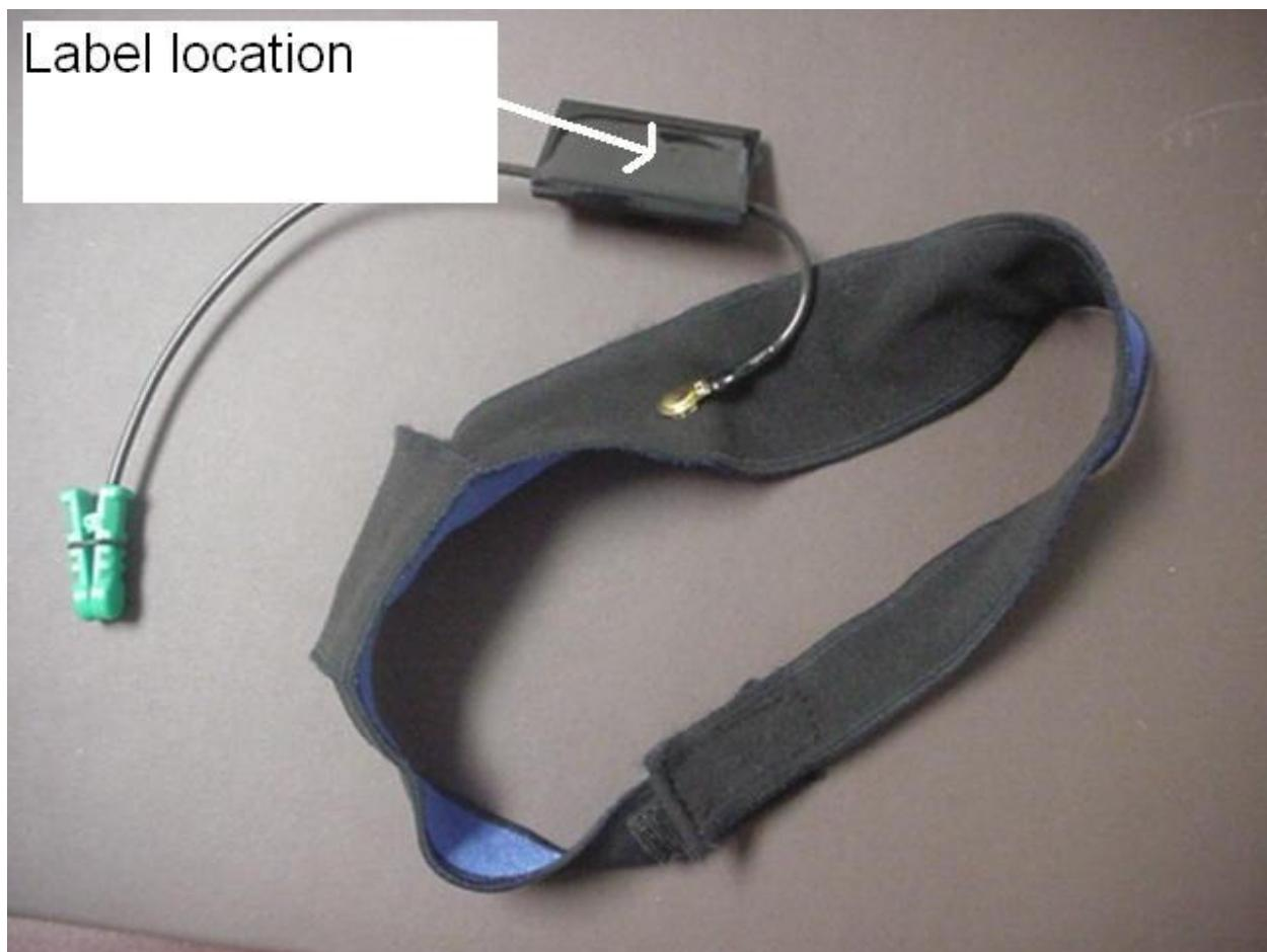
EUT Removed from Headband and Turned over Revealing Flat Bottom
