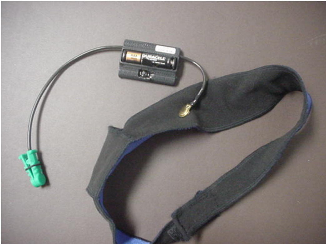
EUT Removed from Headband Sleeve with Battery and On/Off Button Visible
