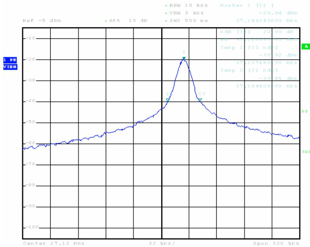
**The results: The unit does meet the FCC Part 15 C Section 15.215 requirements**
