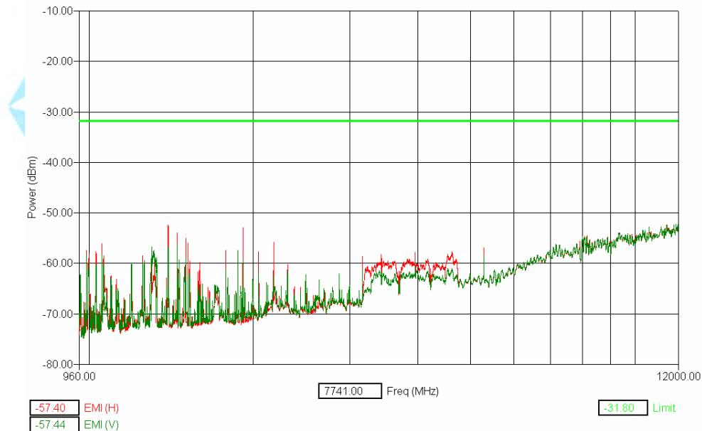
Terminated antenna port measurements made with 1 MHz RBW / 3 MHz VBW at 1 meter distance
