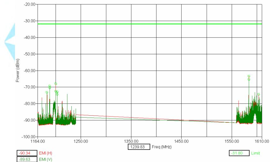
Measurements made with 10 kHz RBW / 10 kHz VBW at 1 meter distance.
