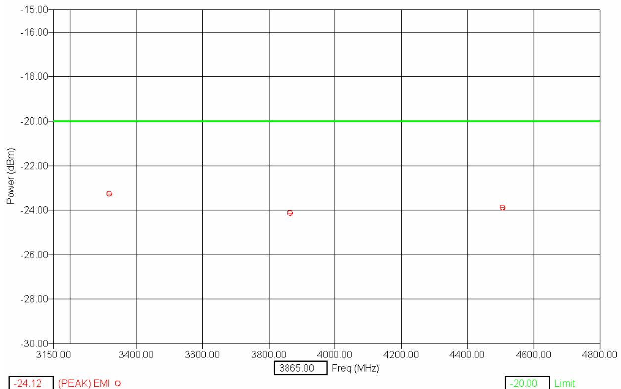
Measurements made with 5 MHz RBW / 5 MHz VBW at 3 meter distance.
