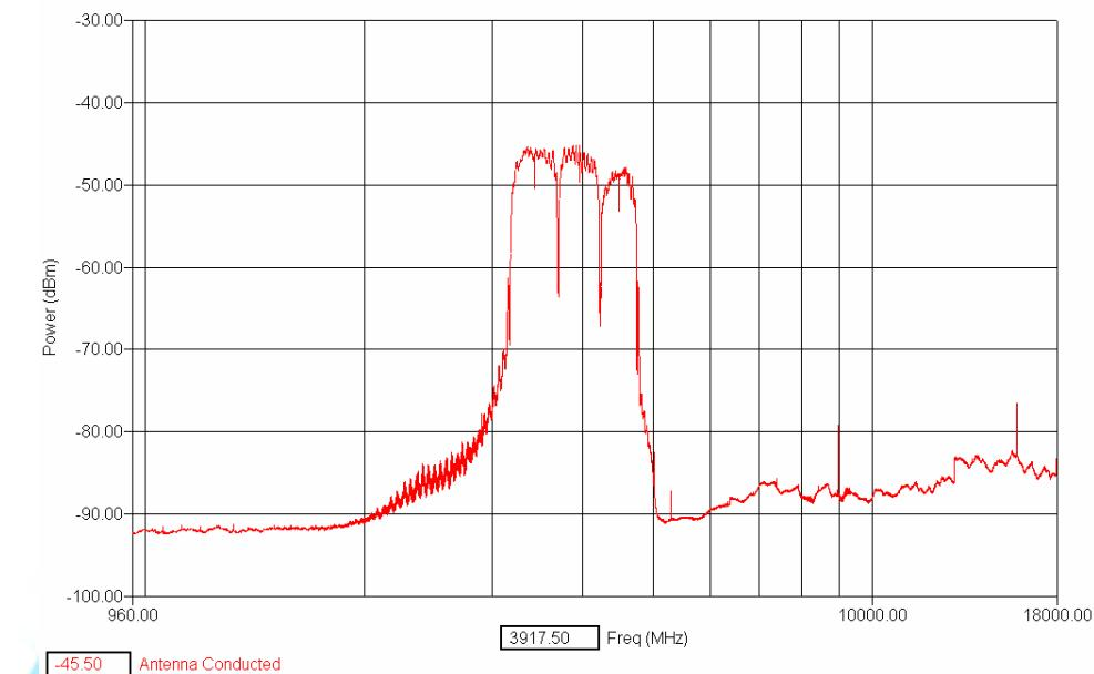
Conducted antenna port measurement made with 1 MHz RBW / 3 MHz VBW
