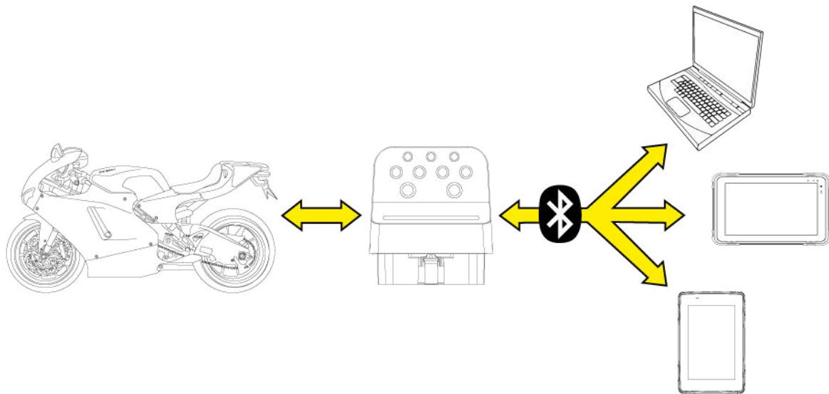
The VCI communicates with the display unit where the diagnostic software is installed via:
