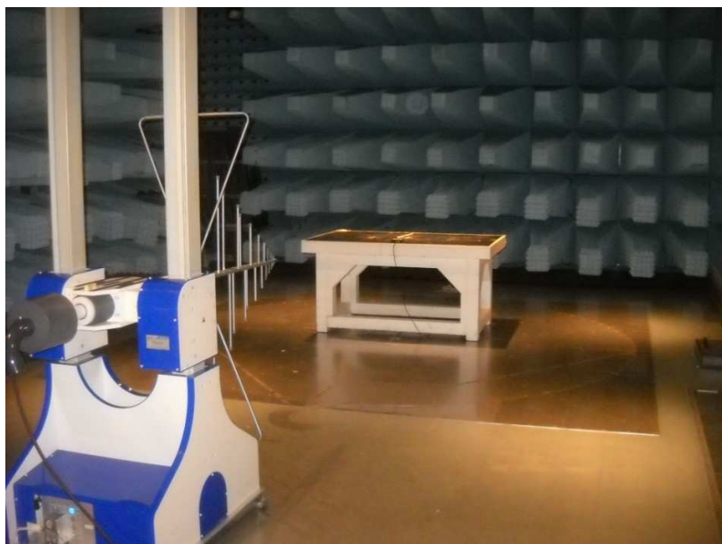
Figure 9.2-1: Radiated emission testing below 1 GHz
