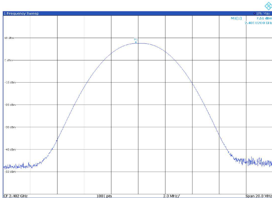
Figure 8.5-1: Output power on low channel
