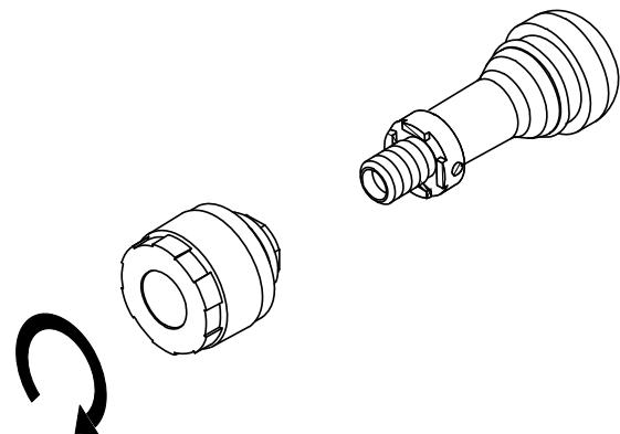
C. Adjust the anti-theft fixed ring position to install it with sensor in place firmly.
