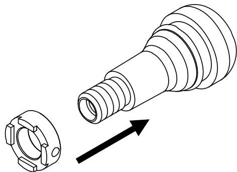
B. Install sensors onto valve stem. Don't install sensors by brute force.
