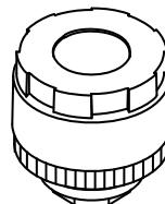
Please refer to “sensor map” to make sure the right position of each sensor and please don't mix up sensor caps either. You will find either sensor cap and sensor body have marks to remind user of its position.
