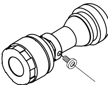
⑤ When four tire pressure sensors are installed, please check with detergent water if the tire pressure sensors and tire valve is completely fitted without any air leakage. (Spread detergent water on the valve stem.)
