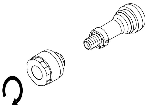
③ Adjust the anti-theft fixed ring position to install it with sensor in place firmly.
