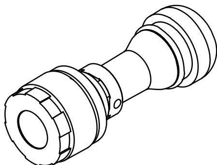
④ Put the hex socket screw onto the anti-theft fixed ring.
