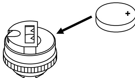
③ Fit sensor cap in a clockwise direction.
