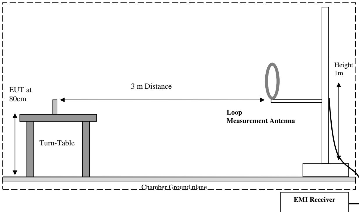
**Radiated Emissions Test Setup 30MHz-1GHz Measurements**
