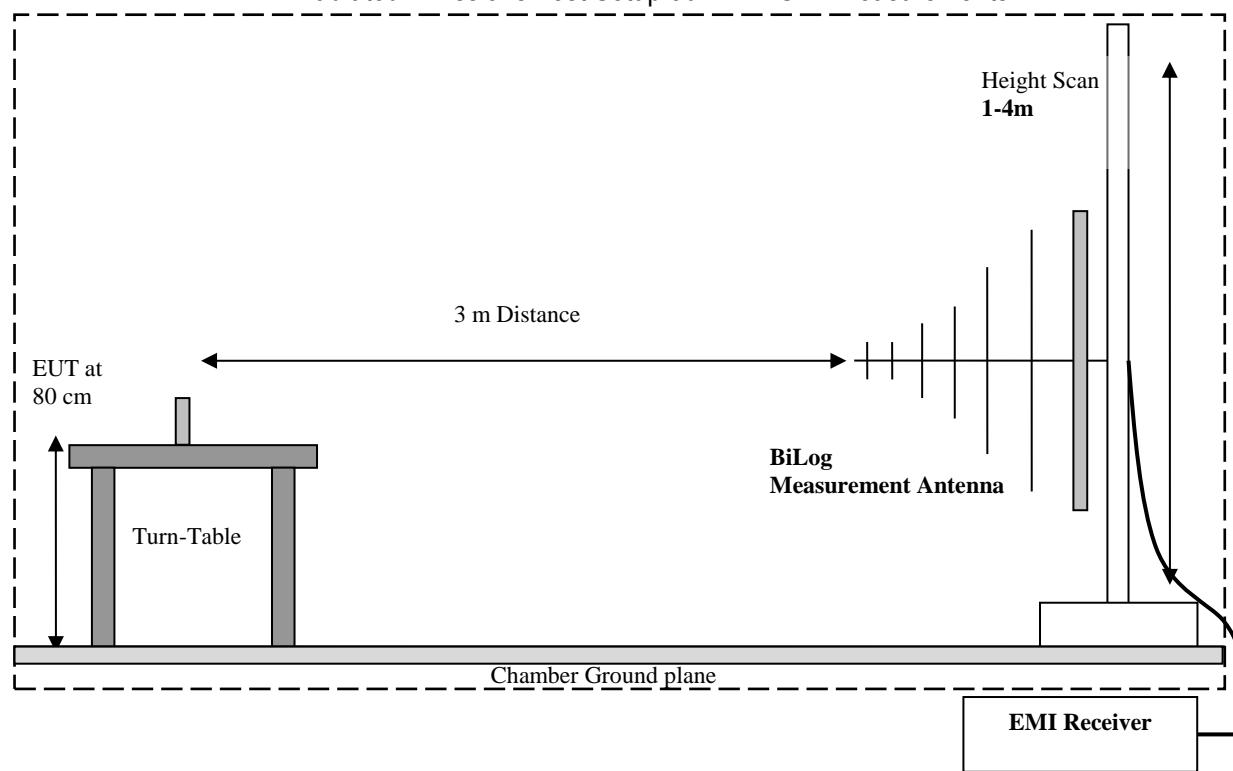
**Radiated Emissions Test Setup above 1GHz Measurements**
