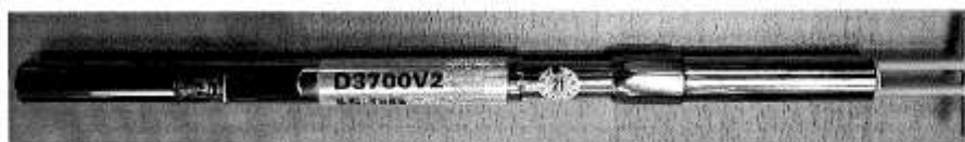
Figure 1 – SAR Validation Dipole
