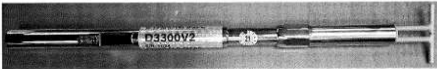
Figure 1 – SAR Validation Dipole
