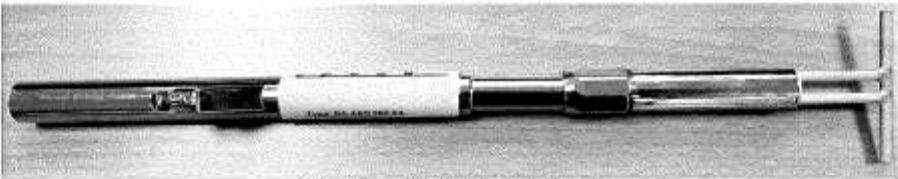
Figure 1 – SAR Validation Dipole
