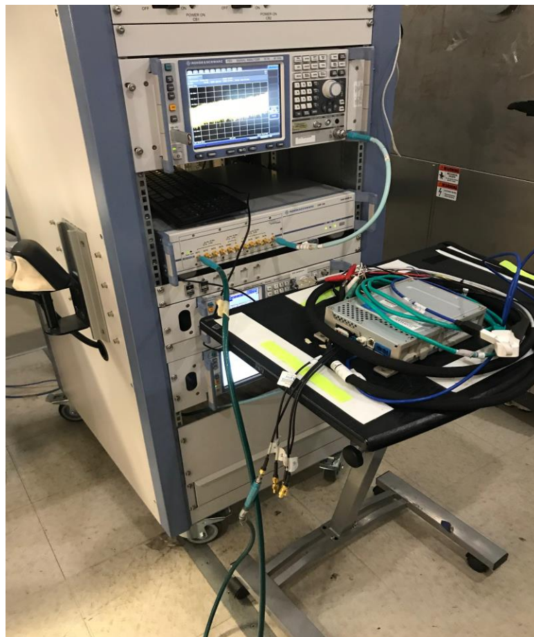
Figure D2: Conducted DUT Set up
