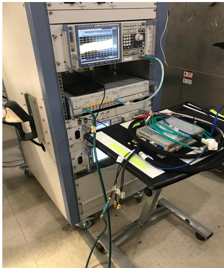
Figure C2: Conducted DUT Set up
