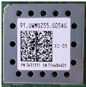
BT/WLAN-Module with shielding plate (20x20mm)
