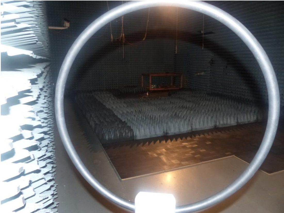
Photo 1: Radiated test setup for H-Field
