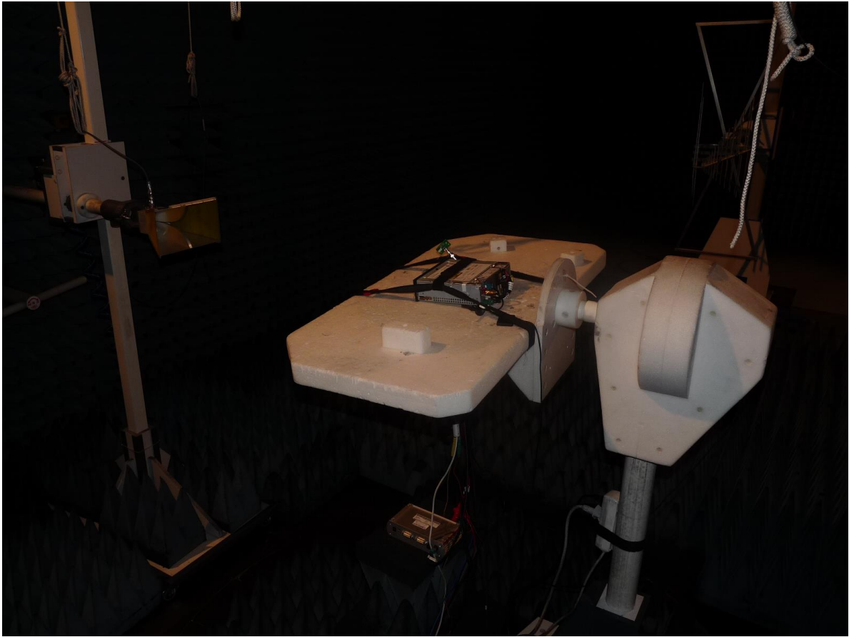
Photo 3: Test setup for radiated measurements (Enclosure, fully-anechoic chamber, 1-18 GHz intentional radiator §15.247)
