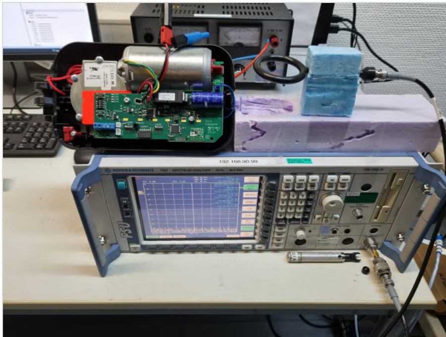
Photograph 9: Test setup conducted measurement of test FW EUT, overview
